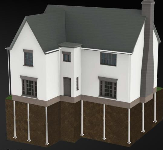
HELICAL PILE SUPPORT SYSTEM FOR HOUSES
