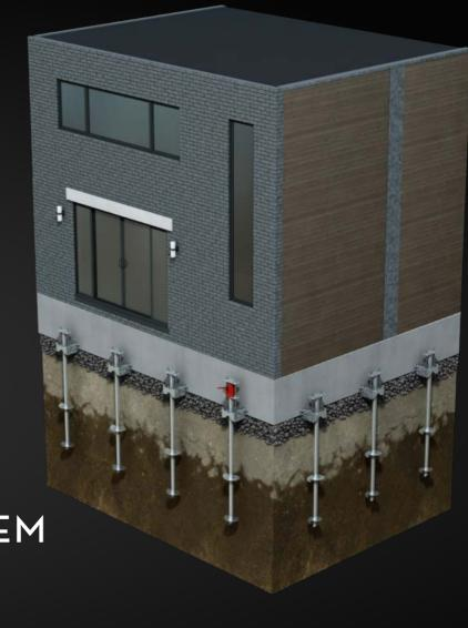
HELICAL PILE SUPPORT SYSTEM FOR FOUNDATION UNDERPINNING
