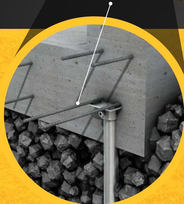
PILE HEAD WITH REBAR
